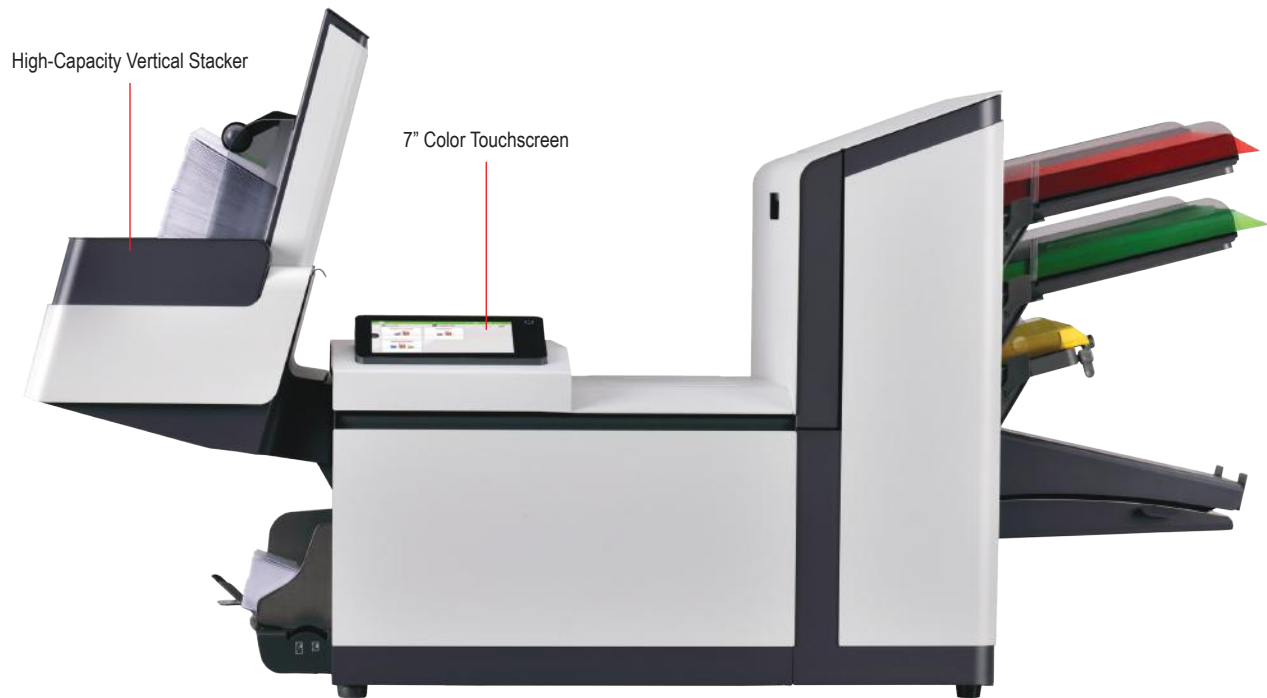
FD 6210-Advanced 2 with new standard High-Capacity Vertical Output Stacker
