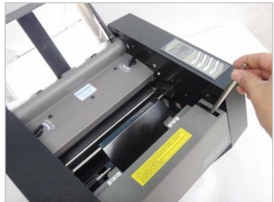
[Insert the tool into the hole on the press roller and rotate the press roller by hand]
